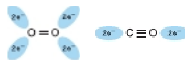
FIGURE 6-4 Orientation of the lone pairs of electrons relative to the O=O and C\equiv O bonds of oxygen and carbon monoxide.
